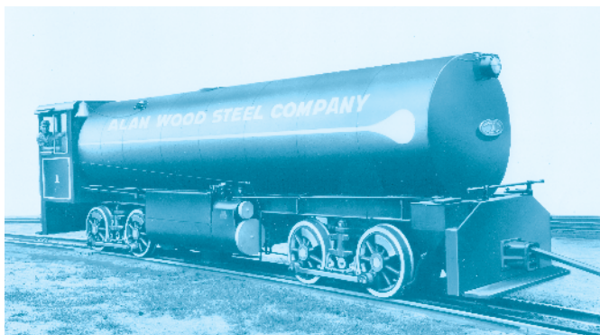
Heisler Locomotive Works built Alan Wood Steel No. 1 in 1940 as a powerful, fireless locomotive able to negotiate the mill's tight curves and clearances. Lake Shore Railway Society
