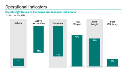
The existing train network now has enough flexibility to absorb the ups and downs and NS could absorb the variables by adjusting train length, train weight and power to keep the trains running to plan. Maintaining power to weight ratios and using more distributed power units to do so was a key factor. And as a result NS moved more freight with fewer resources compared to what that tonnage would have required a year ago.
